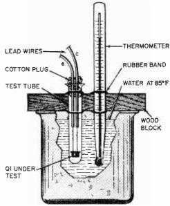
Experimental setup for selecting the best transistor and calibrating the meter in °F.
