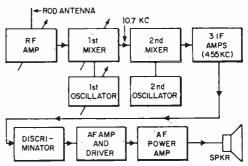
Block diagram of FM receiver for VHF reception. IF's are 10.7 mc. and 455 kc. from 1st and 2nd mixers.
