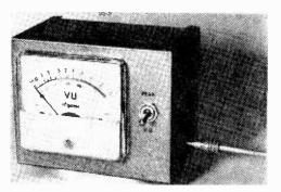
The completed unit gives a professional look to your recording setup. Keep an eye on the meter's pointer when manipulating the tape recorder's volume controls to different levels.
