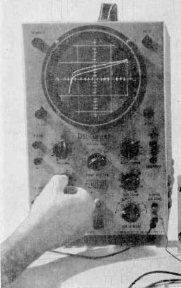
design. The Transistor Characteristics Checker is the unit that will do the trick.
