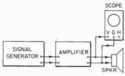
Fig. 19. Audio output from an amplifier can be best rated by observing on 'scope.
