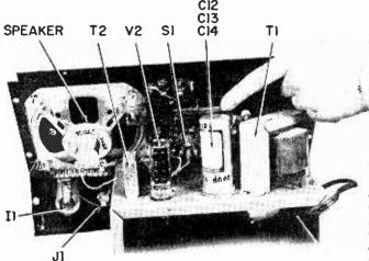
The aluminum chassis is visible when looking into the top of the sloping panel cabinet that houses the receiver. Most of the components, aside from the front panel variable controls and switches, are mounted on the 7"x5" chassis.
