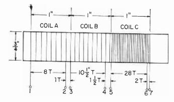
Tuning coil L2 can be wound using this pictorial view as a guide. No. 28 enameled wire is used for all three sections. The turns for each section are spread to cover one inch of the tube. With coil C, the turns will be touching when 30 are wound to the inch.
