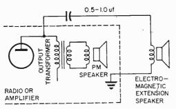
Here, the added speaker is connected in parallel to amp's plate load.
