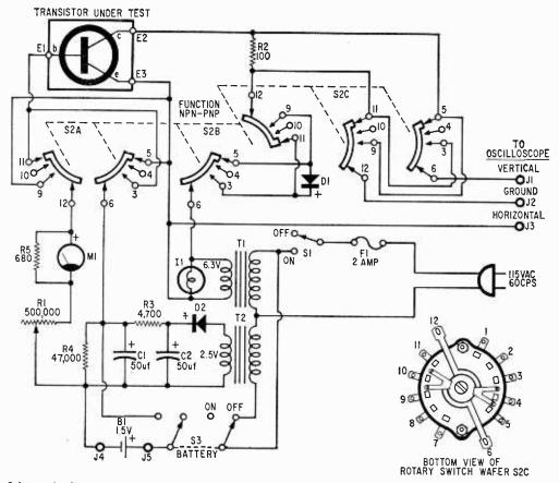
Schematic diagram of Transistor Checker shows switching for checking PNP or NPN transistor.
