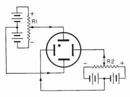
Fig. 6. Position of dot can be varied by adjusting potentiometers R1 and R2.
