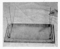
Four threaded rods (above) squeeze the top and bottom of the cabinet together against the sides. To prevent resonances at the joints, an adhesive gasket (below) is used to "insulate" the cabinet sections. The completed assembly will be as rigid as a glued-and-woodscrewed cabinet store-bought.
