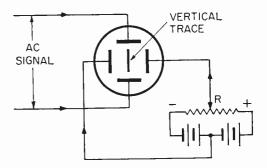
Fig. 7. A rapidly moving AC signal will cause a vertical line trace.
