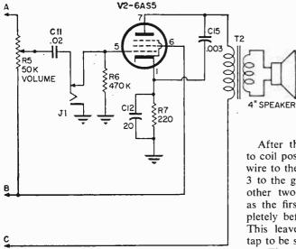
Schematic diagram of receiver shows wealth of circuitry encompassed by 12-pin Compactron.
