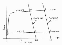
The variation in collector-emitter leakage current of transistor with changing battery voltage and temperature is shown in curves above. Decrease in current between the 1.5and 1-volt points is negligible whereas the current difference with temperature is great.
