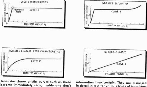
in detail in text for various types of transistors and effect of oscilloscope gain on their shape.
