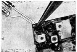
AVOID TOO MUCH HEAT High heat can damage components. Use low heat for soldering, and a pair of long-nose pliers to hold the wire. Pliers act as a heat sink and prevent overheating.
