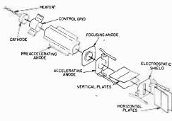
Fig. 1. Electron gun detail drawing.
