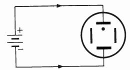
Fig. 4. Dot moves up to positive plate.
