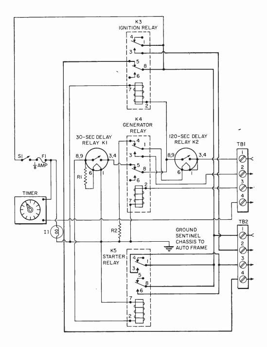
Connections made to terminal boards TB1 and TB2 in chassis box from car's wiring.
