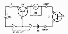
Schematic diagram of the darkroom thermometer shows action of switch S1. It is a D.p.s.t. that removes both batteries from the circuit.
