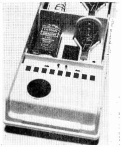
Top photo shows charger ready to charge D and C dry cells once lid has been closed. Below, 9-volt battery is about to be charged.
