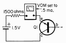
In selecting the best transistor for use as a temperature sensor, a VOM is used to find the transistor with optimum leakage current.
