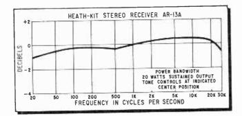
The power bandwidth curve for Heath-kit AR-13A shows less than 1% variation in the listening spectrum with each channel driven simultaneously at full 20-watts by sinusoidal input.
