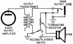
Fig. 3. Typical recorder output circuit. Note terminating resisitor is lifted when the speaker output jack is used. On some models the bottom of the resistor is connected to the top terminal of the jack and is never disconnected.
