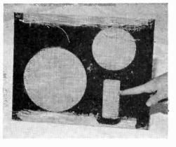
Finger indicates pre-cut tweeter opening in the front panel (above). The smaller of the two round cutouts is for the ducted-port tube. Typical of the wingnut-bolt assembly used by Electro-Voice, the bolt passes through the speaker mounting holes into a captive nut in the front panel as shown in the photo below.
