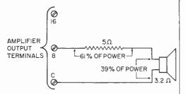
Simple method for connecting one 3.2-ohm loudspeaker to 8-ohm terminals.
