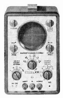
Fig. 12. The EICO 435 oscilloscope, made from a kit, is typical of many models available at moderate prices.
