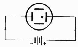
Fig. 3. Dot moves right to positive plate.
