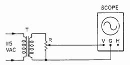
Fig. 14. Set-up for observing 60-cycle AC.
