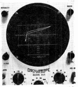
Oscilloscope trace, running from left to right, indicates the transistor under test is a PNP.
