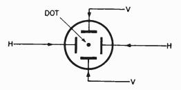
Fig. 2. Undeflected dot (electron stream).
