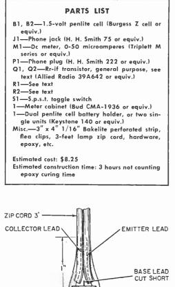
Meter deflection is recalibrated in °F. Lead for Q1 can be cut to any convenient length.
