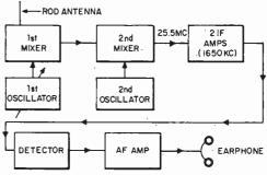
Block diagram of AM receiver for reception in 118-134 mc. aviation band. IF's are 21.5 mc. and 1650 kc.
