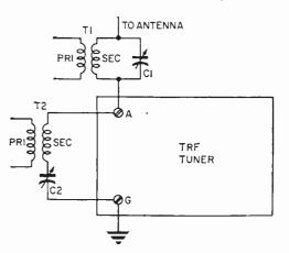
Use Meissner part No. 14-1072 or equivalent for RF coils T1 and T2. Mica trimmer capacitors C1 and C2 are 25-280 mmf. units like Lafayette part No. 34G6832.
