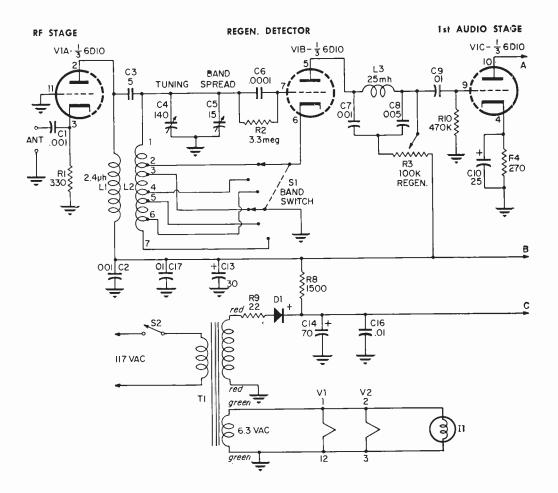
coil wound in a single layer on a plastic tube  $\frac{3}{4}$  inch in diameter. Coil A has a total of 9 turns of No. 28 enameled wire tapped at the 8th turn for terminal 2 that goes to the cathode circuit. Coil B has a total of 12 turns tapped at the  $10\frac{1}{2}$  turn. Coil C of the 40 to 80 meter band is 30 turns tapped at
