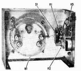
Note the meter has two sets of terminals. Extra set is the power connections for the panel lamps. If the meter is inoperative, connection has probably been made to the lamp terminals. Special bracket holding potentiometer R2 is standard stock; it can be made from aluminum scrap.
