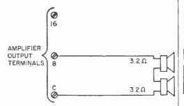
Two 3.2-ohm loudspeakers in series can be connected across 8-ohm terminations.
