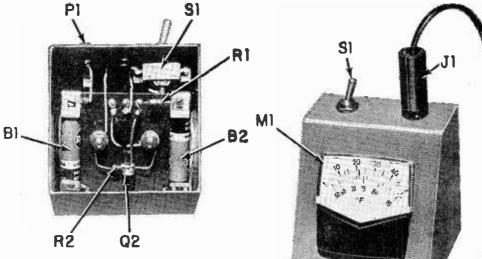
Darkroom thermometer components fit comfortably in a meter case. Note the bakelite mounting board is held by meter terminals.
