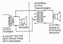
An universal output transformer is the best method for matching an add-on loudspeaker. Adjust taps for best sound.
