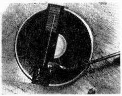
tracking is readily apparent. The mounting position that produces the minimum amount of movement on the scale is the proper positioning for greatest fidelity with the particular tone arm and cartridge being tested. Tru-Trak is precision made from Lucite, fits standard cartridge mounting and can be installed in minutes—price is \$6.95 postpaid. (For more information write to Alard Products, Dept. TE72, Somerset, California. 95684.
